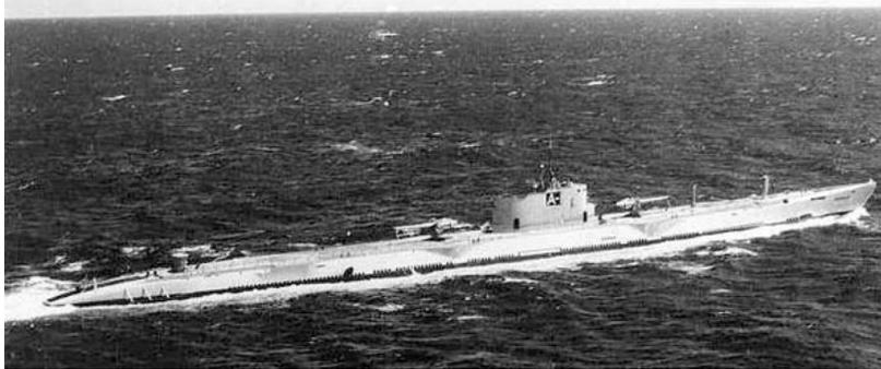
Originally named V-4, Argonaut was commissioned in 1928. At the time, she was the largest submarine in the U.S. Navy, a distinction she retained until the advent of nuclear submarines in the 1950s. Designed as a minelayer, Argonaut was 385 feet long and displaced 2,710 tons (4,080 submerged), with 4-21" torpedo tubes, and two mine laying tubes aft. As originally configured, 60 mines were carried. She also carried a pair of 6"/53-calibre deck guns, one forward and one aft.
